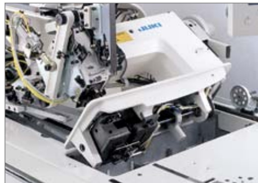
Maintenance works are conducted with the machine head tilted.
